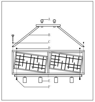
STEP 2:Weave the fixture wire through every 3rd link in the chain and canopy. Connect the chain to the bottom loop on fixture and top loop on canopy.
